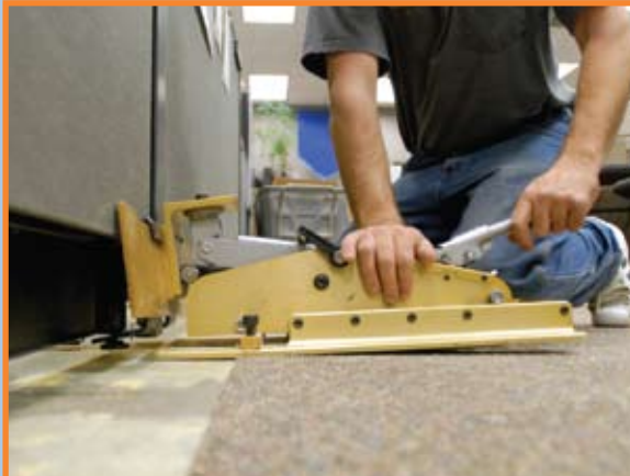
Mini-lift equipment is inserted under work stations.
